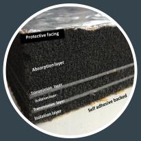
Pyrosorb-S in combination with DS5 dampening sheets, glass cloth heat resistant top layer and self adhesive backing
